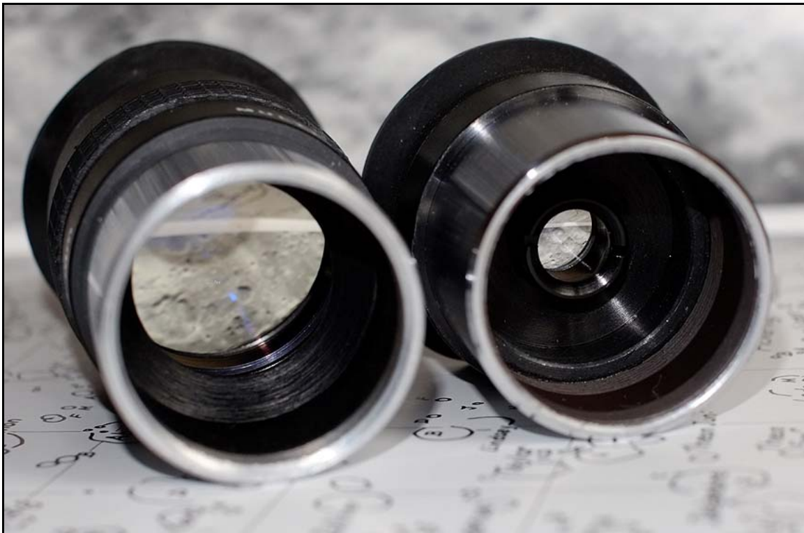
Figure 2. Interior view of the 25mm (left) and 10mm (right) TAL Super Plössls Image by the Author; Eyepieces courtesy of www.talteleoptics.com
