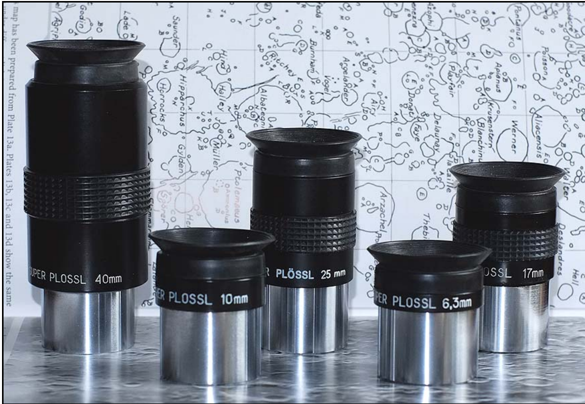
Figure 1. 6.3mm, 10mm, 17mm, 25mm, and 40mm TAL Super Plössls Image by the Author; Eyepieces courtesy of www.talteleoptics.com
