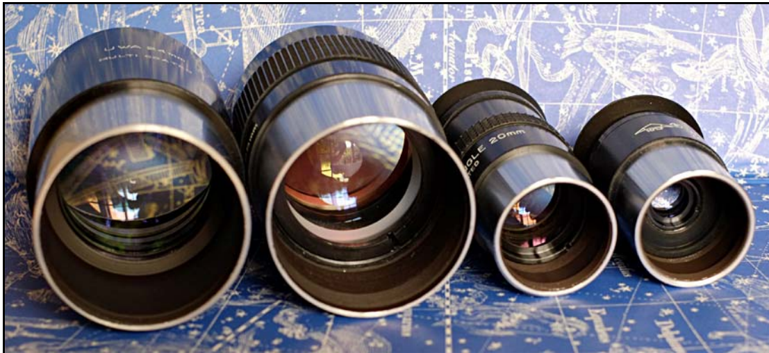
Figure 3. Interior views (left-to-right) of the 24mm UWA, 25mm UWA, 20mm SWA, and 10mm SWA Image by the Author; Eyepieces courtesy of www.talteleoptics.com
